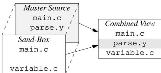
In this environment, the sand-box has the same tree structure as the project master source. This allows developers to safely change things across separate modules, e.g. if they are changing a module interface. It also allows the sand-box to be physically separate – perhaps on a different disk, or under their home directory. It also allows the project master source to be read-only, if you have (or would like) a rigorous check-in procedure.
